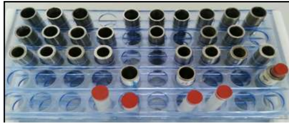
FIG. 3. A photo of lead shield tubes and samples.
